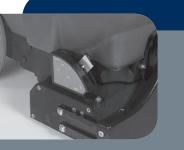
Brush adjusts to eight cleaning positions for maximum performance and a storage position increases brush life.
